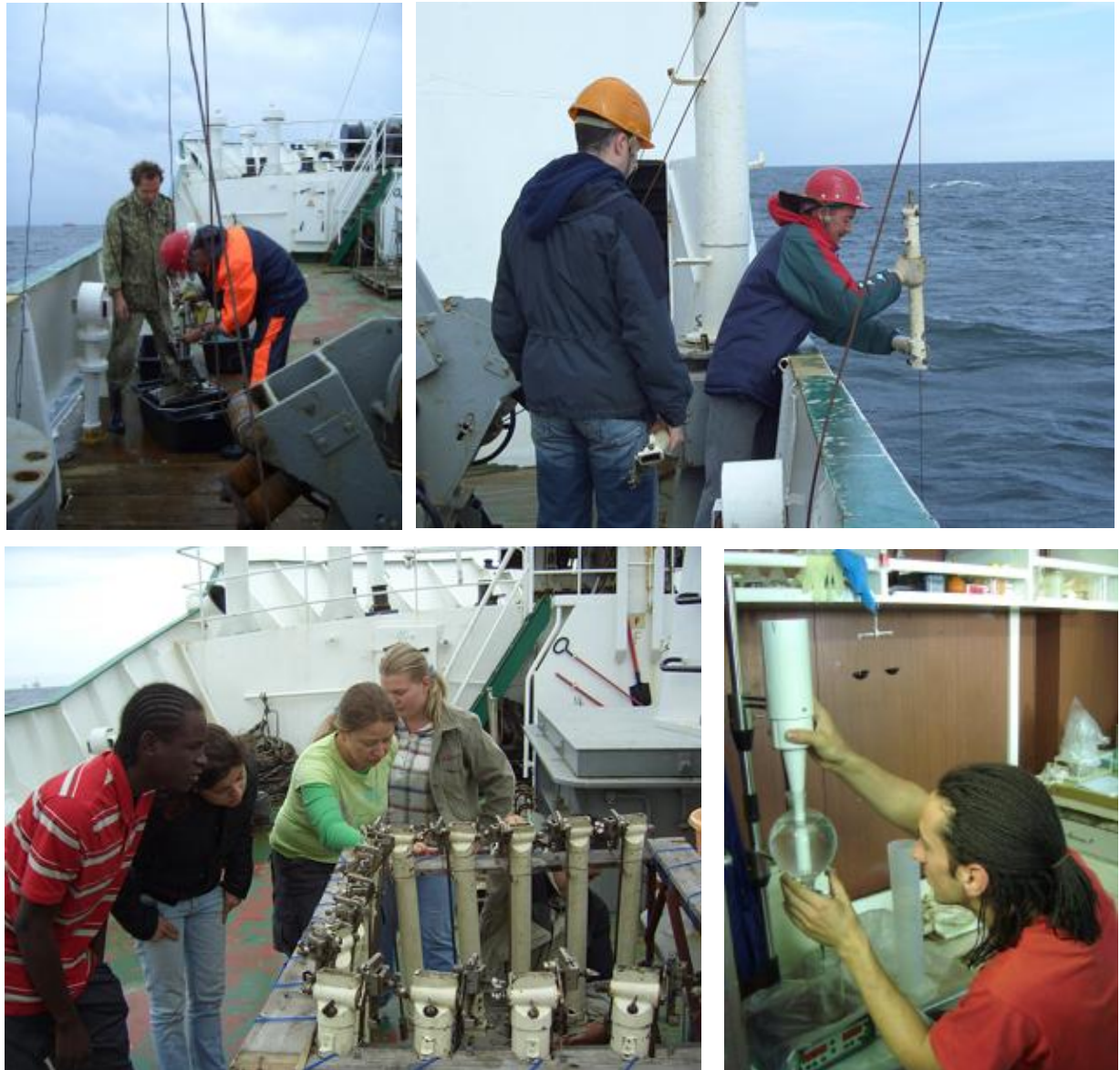
Figure 5. Routine work on a complex oceanographic station (from left: taking samples of bottom sediments; work with sampling bottles; teaching students to take water samples; work in a chemistry lab)
